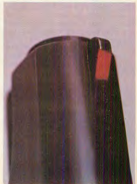
Below: Baughman type "quick-draw" front sight with Red insert was opted for by author Taylor. Sight is silver soldered, rather than pinned, for optimum reliability.
